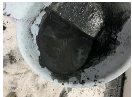
Figure 8: Hand-made slurry of silica fume
