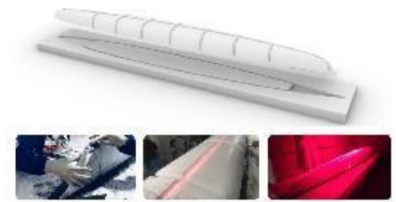
Figure 10 : The combination of male and female molds with infrared positioning
